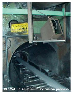
The **IS 12-AI** is a special development of the well proven IS 10-AI for aluminium applications in temperature ranges between 350 and 1050°C.
